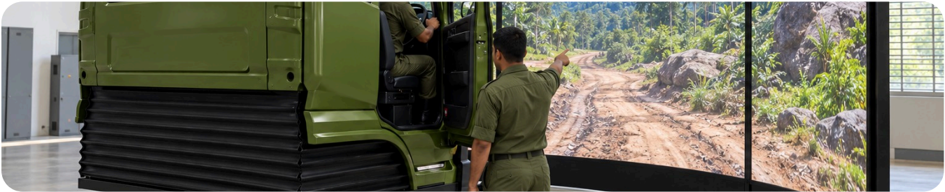
Illustration: military driver training, with the curved screen wrapped around the cab.
