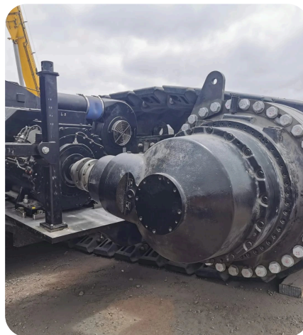
Installing the crawler propel drive: motor and planetary gearbox.
