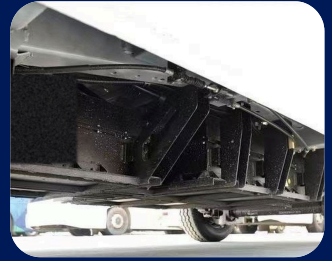
CATL battery under the floor
