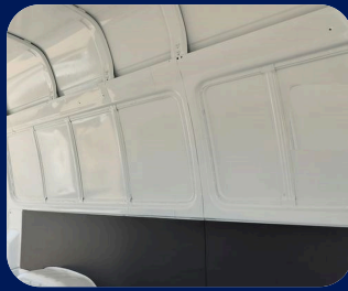
Lined walls and floor
