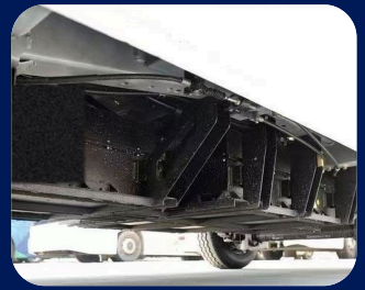
CATL battery under the floor
